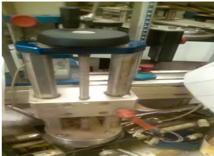
Figure 2: Closer View of Hand wheel for upward and downward motion of Labelling head for vertical orientation Label Adjustment
